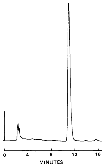
Figure 6 —HPLC chromatogram of erythromycin ethyl carbonate on \mu -Bondapak C 18 at 70°. Mobile phase: acetonitrile-0.2 M ammonium acetate-water (60:10:30) at pH 7.0.
